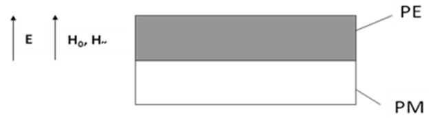
Figure 1. Schematic of the layered composite structure for longitudinal case.
