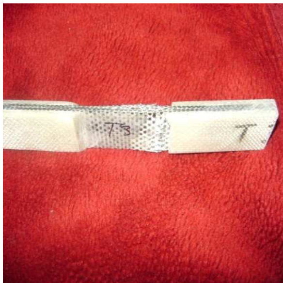
Fig 8. Failure of Tensile Specimen
