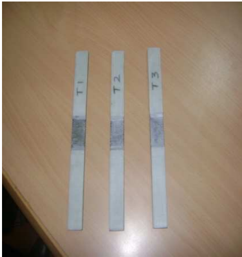
Fig1. 0^\circ/90^\circ Angle ply laminate
