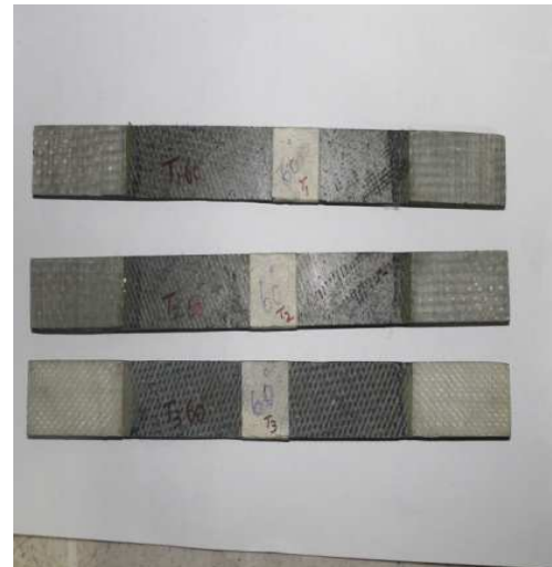
Fig 3. 60^\circ/30^\circ Angle ply laminate
