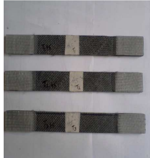
Fig 2. 45^\circ Angle ply laminate
