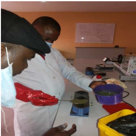
Figure 3.5. Composites Lamination in Progress.
