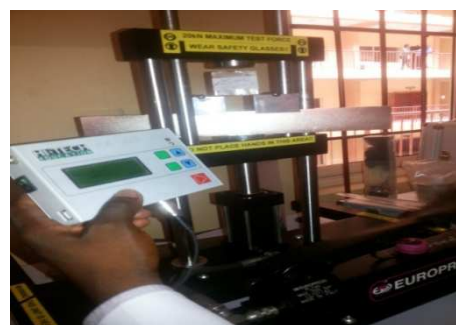
Figure 3.11. Tensile Property measurement in Progress.
