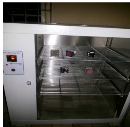
Figure 3.10. Conventional Oven Curing in Progress.
