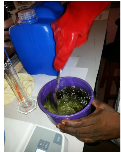
Figure 3.4. Mixing of the Composites in Progress.
